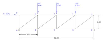
check out the free-body diagram (reactions removed and replaced with force vectors)
